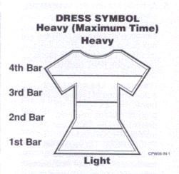
The preset factory soil level setting is the lowest time limit under the **2nd Bar** column in the table above (the first and second bars of the dress symbol will be lit).
